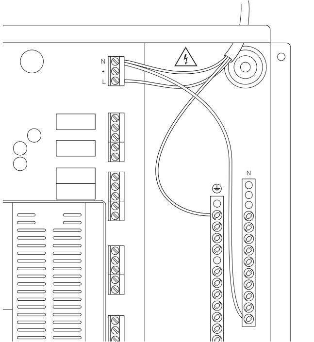
! Refer to product label for Earth Bar and Neutral Bar wire gauge and torque ratings.
