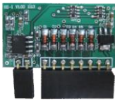
BZ-I Dry contact input card (for connecting with a Technical parameters third-party panel)
