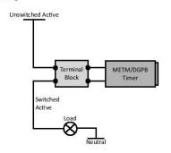
The terminal block included with the timer should be used to carry out the electrical connections, as shown below.
