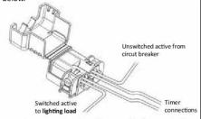
Once the connections have been made, the terminal cover should be snapped closed to ensure the screw terminals are not exposed.
