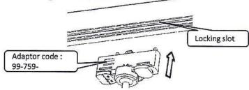
Right knob, turn clockwise 90° to connect to the (N – neutral) circuit of the track.
