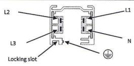
• To mount the adaptor into the track system. Check and ensure both knobs are in the open position as below shows.
